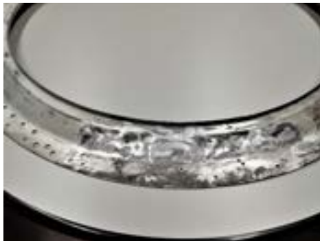
Figure 4. Component cold sprayed and grinded
